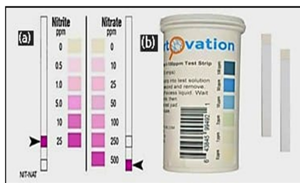
Fig. 3. Strips used to measure the \text{NO}_2 , \text{NO}_3 , and \text{H}_2\text{O}_2 concentrations in ppm.
