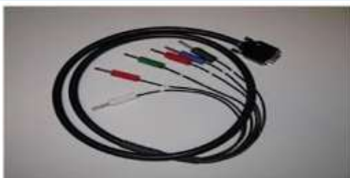
Figure 3-6-interface cables between electrodes and the device
