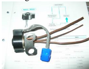
Figure 3. Proportional Control Valve
