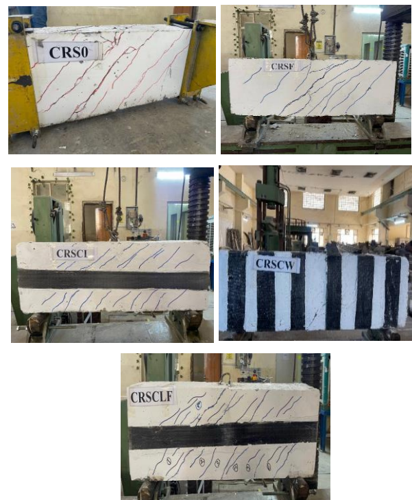
Figure 3. Failure modes and cracking patterns of all Deep beam Specimen
