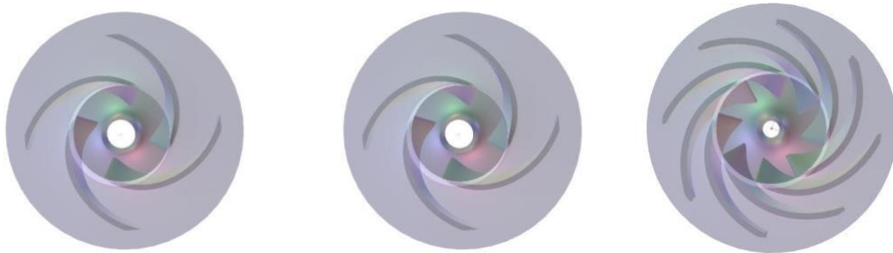
Figure 4: Shows impellers with varying numbers of blades: (a) blade number four, (b) blade number six, and (c) blade number eight.
