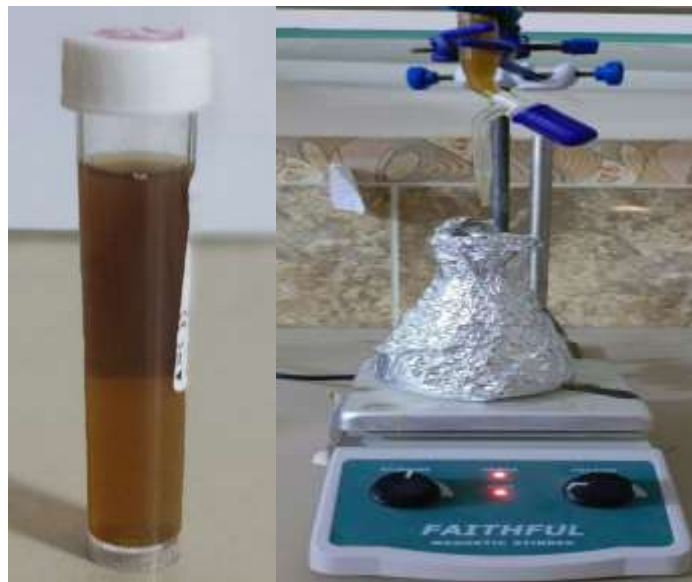
Figure 12: Mint extract with silver nitrate during the calibration process
