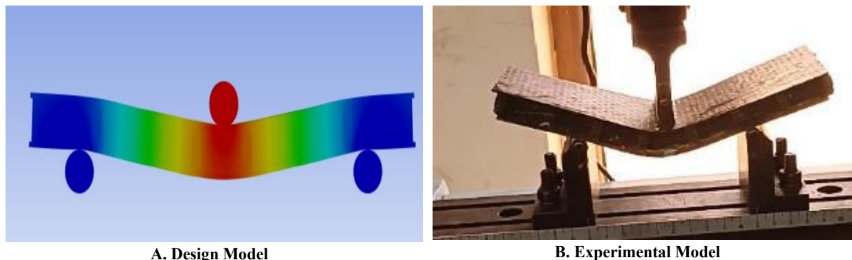
Figure 6: A) Numerical design model under 3-point bending, B) Experimental sample test under 3-point
