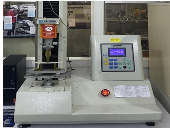
Figure 6: Universal testing machine for flexural testing
