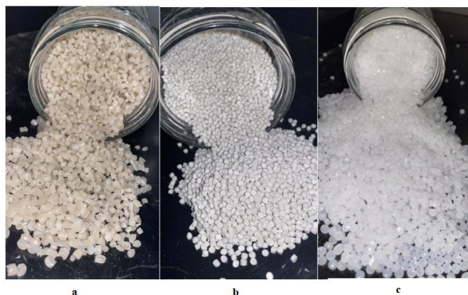
Figure 1: Materials used: (a) recycled plastic; (b) \text{CaCO}_3 filler ;(c) HDPE
