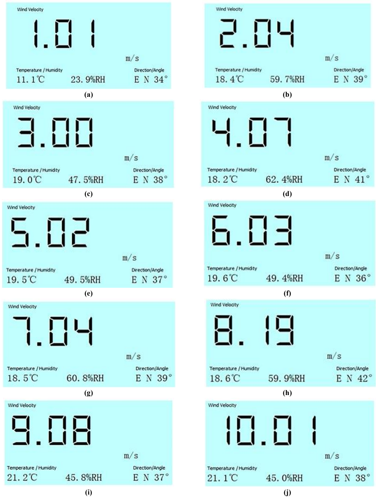
Figure 9: Air flow velocity measured by varying the rotation of the fans (a) air flow at 1 m/s (b) air flow at 2 m/s (c) air flow at 3 m/s (d) air flow at 4 m/s (e) air flow at 5 m/s (f) air flow at 6 m/s (g) air flow at 7 m/s (h) air flow at 8 m/s (i) air flow at 9 m/s and (j) air flow at 10 m/s
