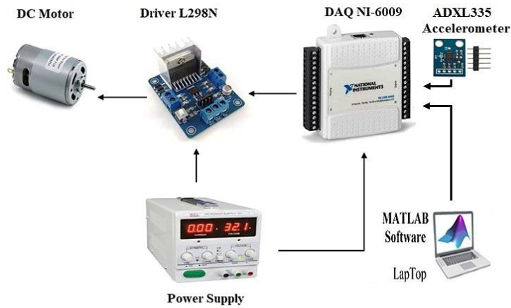
Figure 7: Output rotational speed generation process through L298N and power supply
