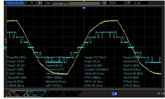
Fig. 3. Inverter output synchronized with the grid.
