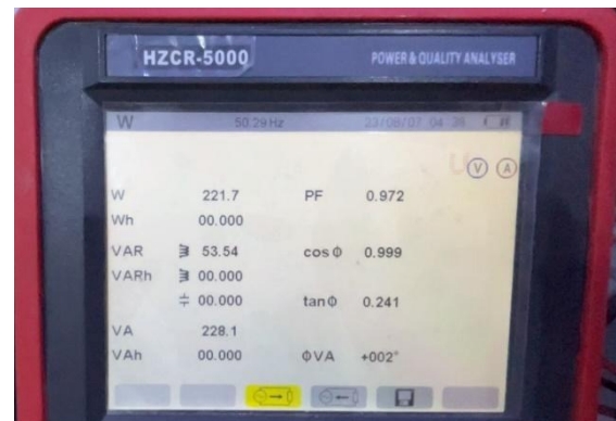
Fig. 5. Power analyzer measurements during 1 A active current injection.
