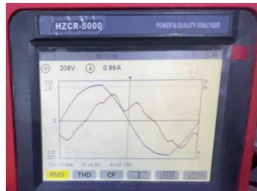
Fig. 8. Waveform of reactive current injection at 1 A using fuzzy logic control.
