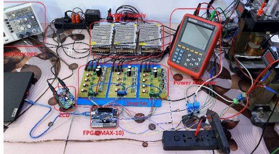
Fig. 1. Experimental setup of the proposed fuzzy logic-controlled grid-connected inverter.
