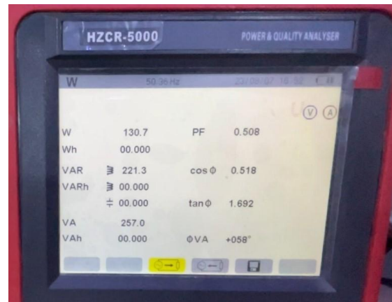
Fig. 9. Power analyzer measurements during 1 A reactive current injection.
