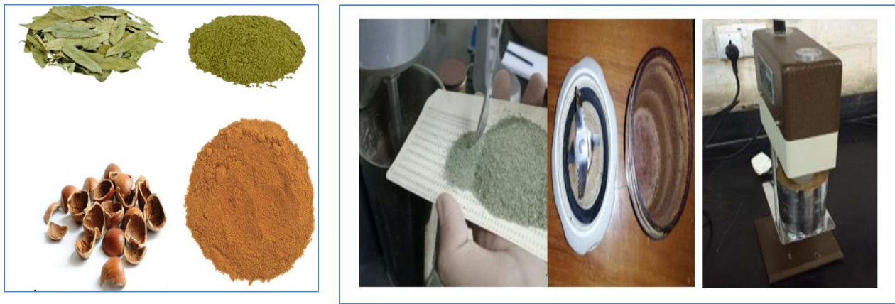
Fig. 2 The used materials Ground Hazelnut Shells and Willow Decoction and experimental work in the laboratory.
