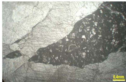
Fig.9: Calcite syntaxial vein fill (ppl) (see Fig.18)
