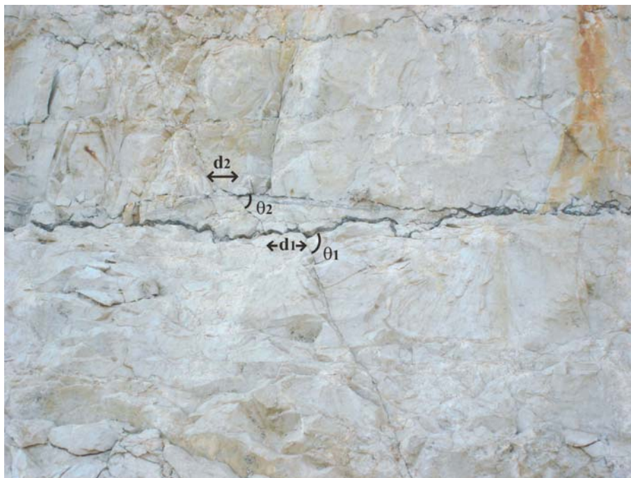
Fig.19: Previously continuous vein, segmented by pressure-solution surfaces
