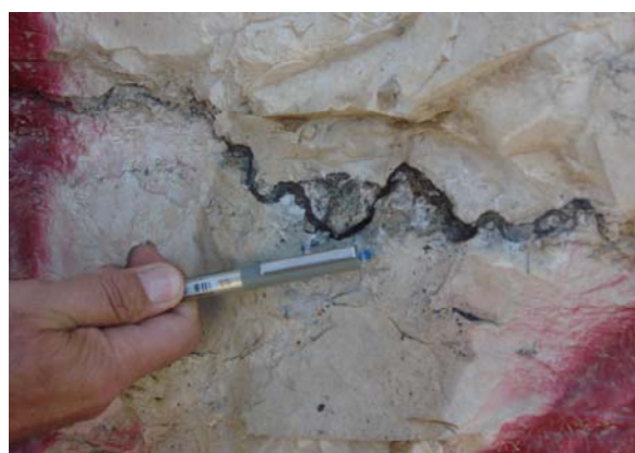
Fig.6: Pyrite nodules along stylolite seams
