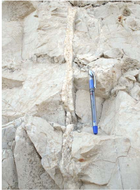
Fig.18: Orthogonal syntaxial vein with fibrous calcite fill
