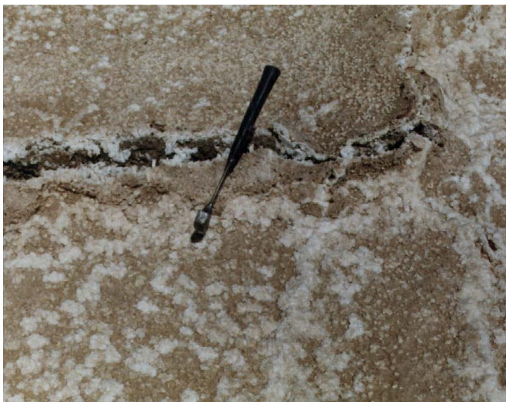
Fig.6: Recent and older salt crusts along cracks
