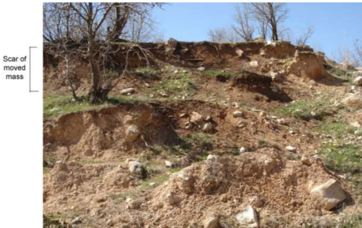
Fig.13: Soil slump shows the scar of moved mass in the Station No. 14 (Photo direction is 230^{\circ} )
