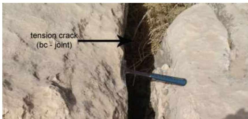
Fig.11: Tension crack represents bc-joint, is an indication of instability in the Station No. 2 (Photo was taken above the bedding plane)
