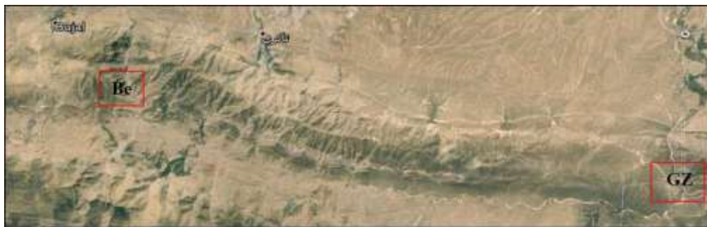
Fig.39: Google Earth image (facing south) of Aqra anticline. Note the absence of Wine glass feature and presence of two water gaps, Bekhme (Be) and Gulley Zanta (GZ)
