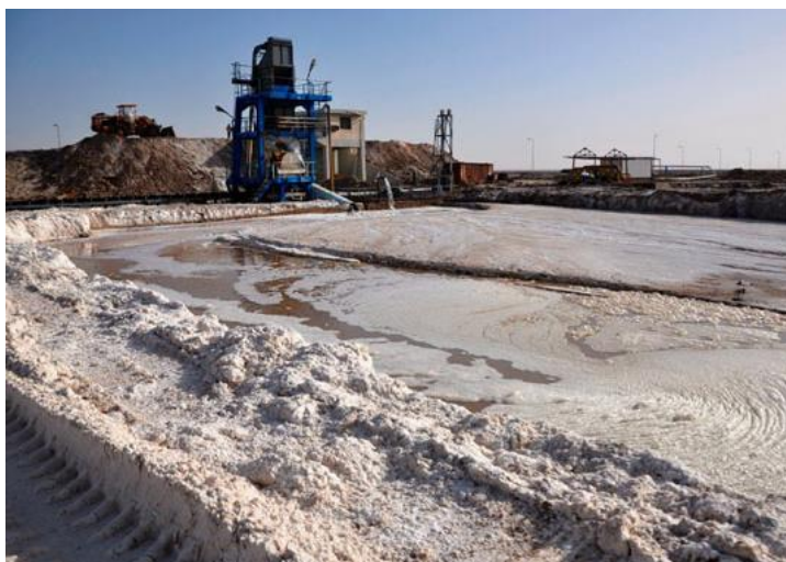
Fig.8: Salt washing at the Samawa Salt Plant
