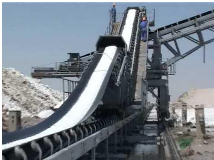
Fig.9: Salt transport by conveyor belt for stacking at the Samawa Salt Plant
