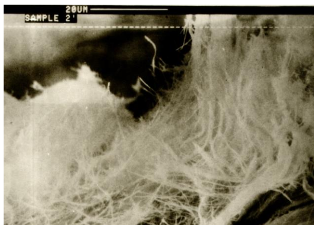
Fig.3: SEM image showing well developed fibres of palygorskite in Jabal Maqlub fracture-fill deposits (after Al-Bassam et al. , 2000b)
