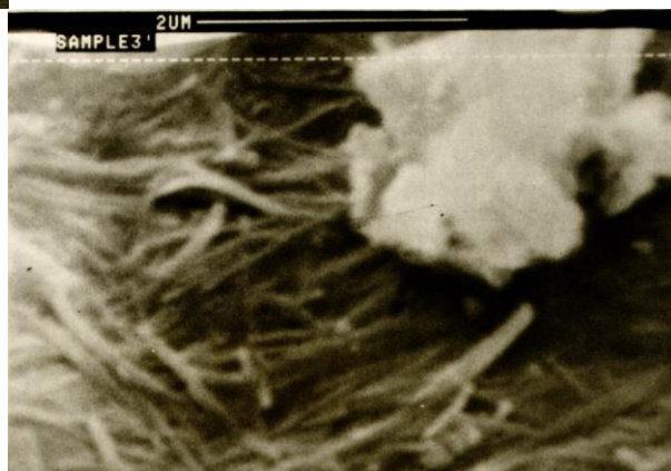
Fig.4: SEM image showing palygorskite fibres in the Safra Beds (after Al-Bassam et al. , 2000b)
