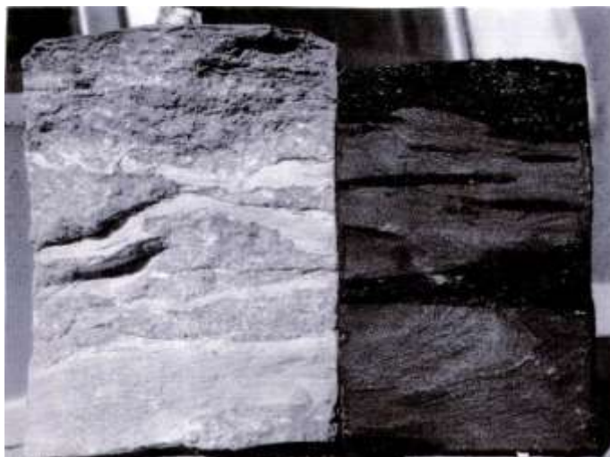
Fig.12: Phosphorite-shale association, Left: oxidized by weathering (light color) Right: original unoxidized (dark color)
