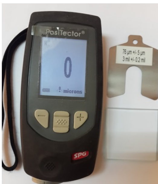
Fig.2: PosiTector device with standard plate and glass for the device normalization used for measuring the surface roughness
