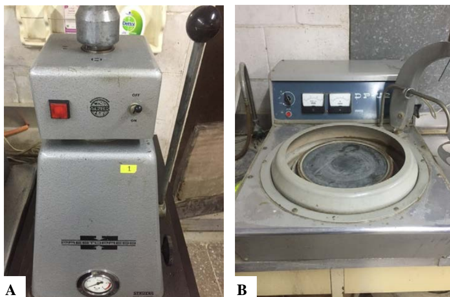
Fig.1: Presto-press device (A) used for making polished section; Dp-U2, a rotary grinding and polishing machine disc (B)
