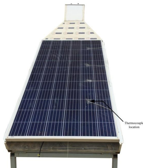
Fig. 2.Photo of the experimental set-up for PV cell with air guides cooling system.
