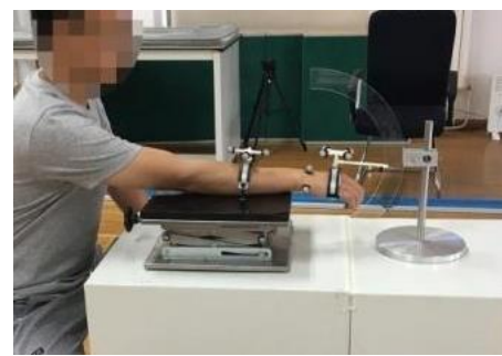
(b) Wrist radial-ulnar rehabilitation module.
