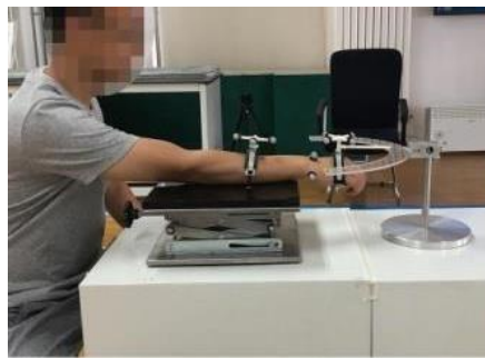
(a) Wrist flexion-extension rehabilitation module.
