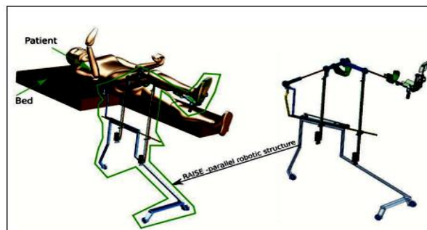
FIGURE 15 3D CAD model of the RAISE robot [30]
