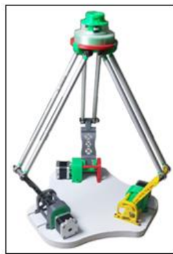
FIGURE 14 3D CAD model of the robot [28]
