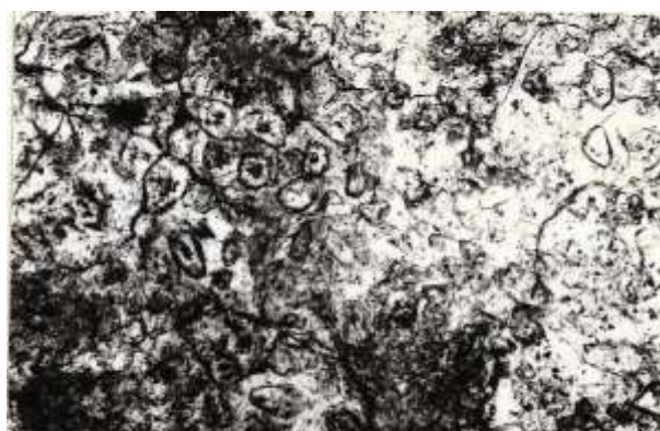
Fig.10: Photomicrograph of the dedolomitized rock from the Jil Formation, Ab-3, at Abou Allum area, Large calcite crystals show poikilotopic texture with dolomite as inclusion or as ghosts of the original dolomite crystals outline. Dolomite rhombs are partially replaced by calcite, especially the outlines. The dark centres of the crystals are usually remained unaltered. Plane polarized light. The dark areas represent clayey lime-mud
