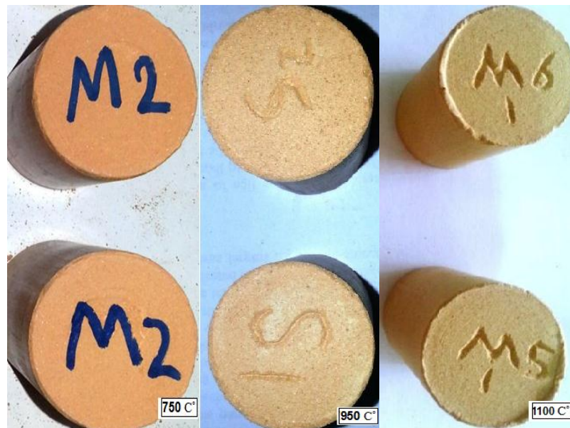
Fig.6: The bricks samples that fired at (750, 950, and 1100) C° by pressing
