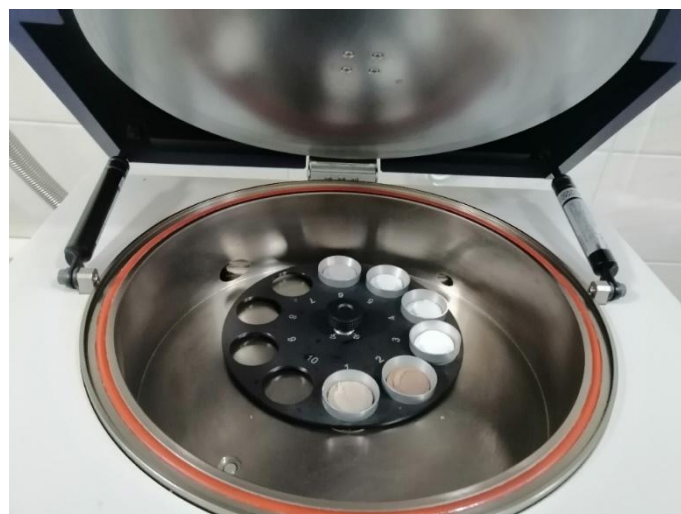
Fig. 5: XRF illustrates the sample chamber.
