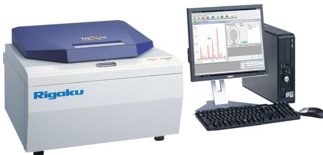
Fig. 4: X-ray fluorescence spectrometry (XRF) Instrument with their computer program.
