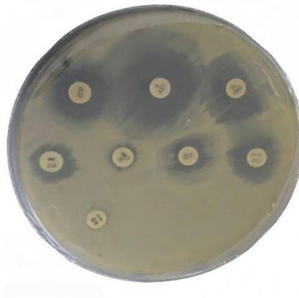
Fig. 4: Antibiotics susceptibility test for the isolated bacteria on agar solidified YEM media.
