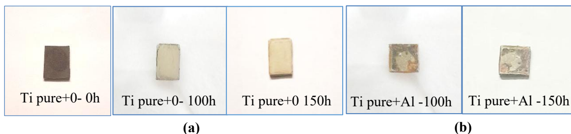
Fig. 13: Surface appearance of pure titanium. (a) Non-metallic. (b) Painful strips at 900°C for 100h and 150h.
