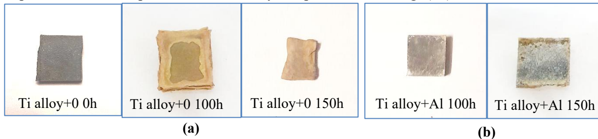
Fig. 11: Surface appearance of two samples of non-painful titanium alloy (a) and (b) painful both at 900°C for 100h and 150h.
