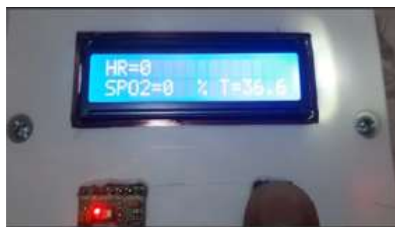
Fig. (12) Display Temperature on LCD
