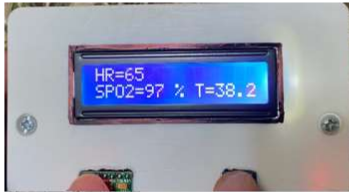
Fig (13) Display Reading of Both Sensor
