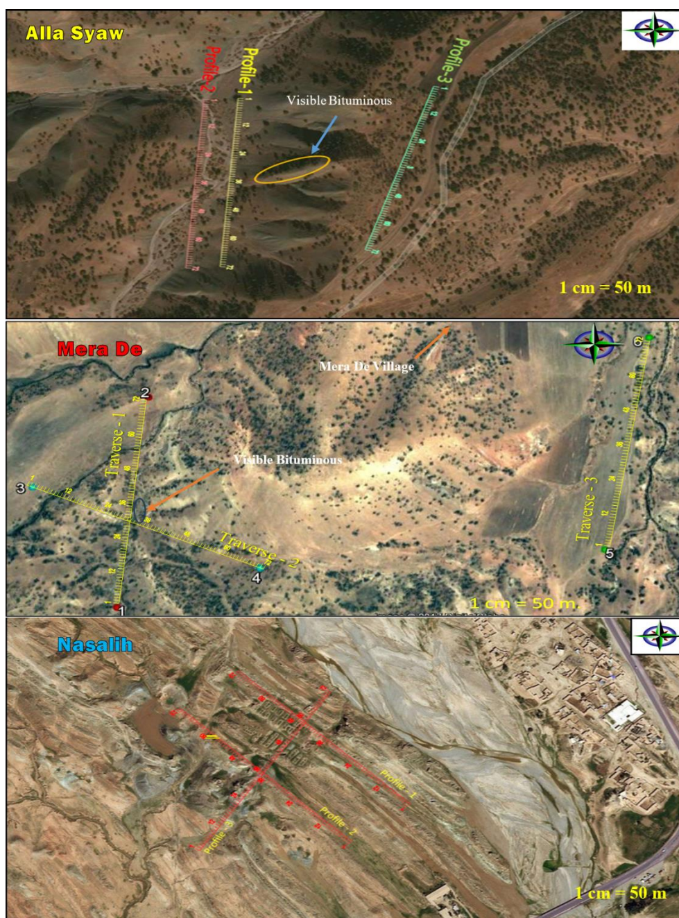
Figure 3: Locations of the 2D Resistivity Imaging profiles in the studied sites.
