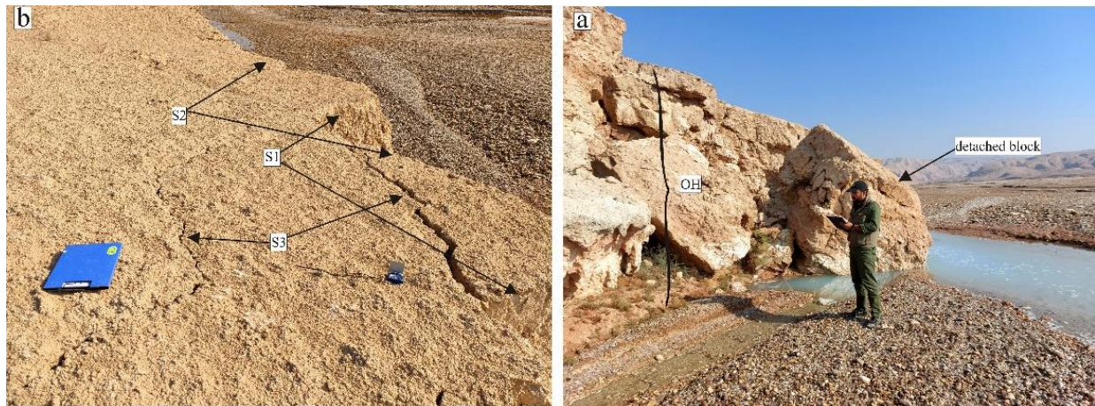
Figure 6: a) Side view showing slope and size of the detached block, b) view showing the three sets of joints.
