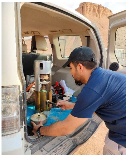
Figure 2: Point load testing for the selected rock samples in the field.
