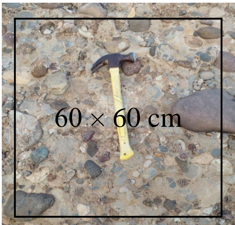
Figure 5: The field photograph shows a 60 cm x 60 cm grid used in the clast count analysis.
