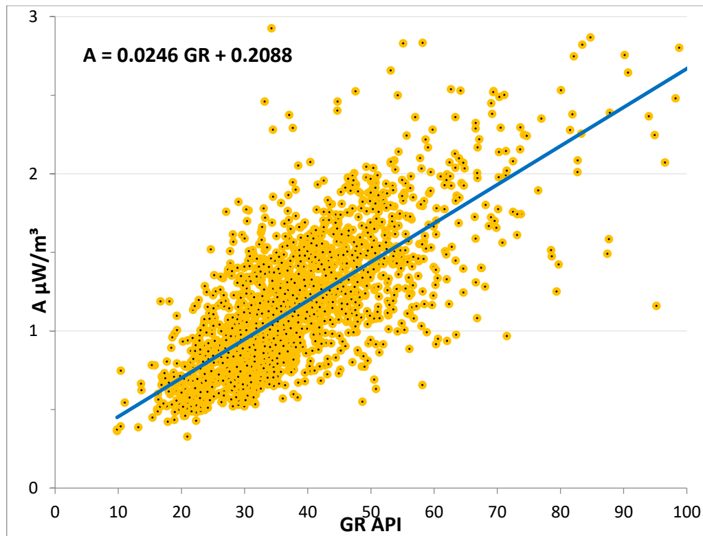
Figure 3. Empirical relationship to determine radioactive heat generation (A) from GR log readings in API units.
