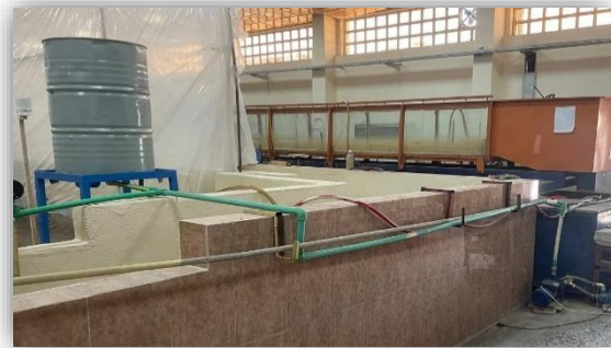
Fig. 3 Cylindrical Tank and Water Supply System.
