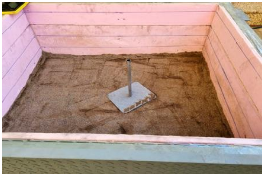
(b) Compacted the soil as layers
