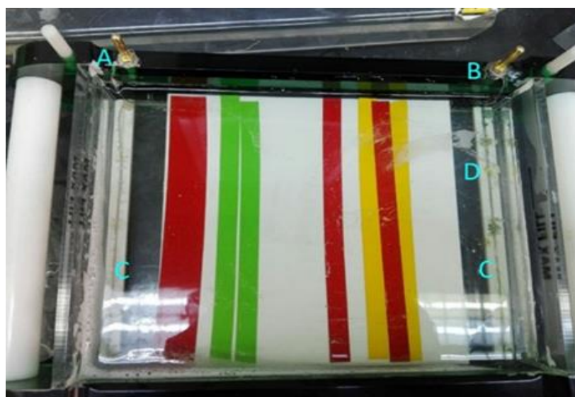
Fig. 1. Stainless steel wire fitted inside the GED tank: A: cathode; B: anode; C: stainless steel wire; and D: silicon glue for wire fitting
