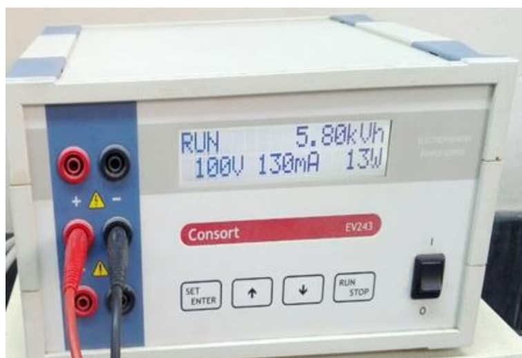
Fig. 3. DC power supply connected to the electrodes of GED with potential difference of 100 V
