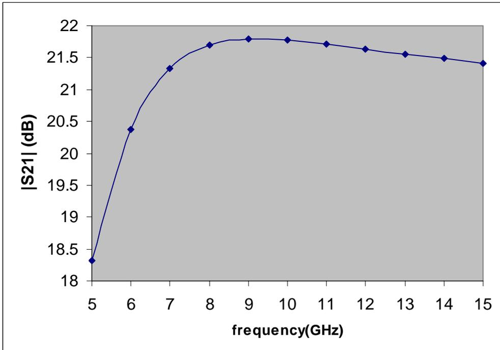
Fig. 3 : TIA gain versus frequency.
