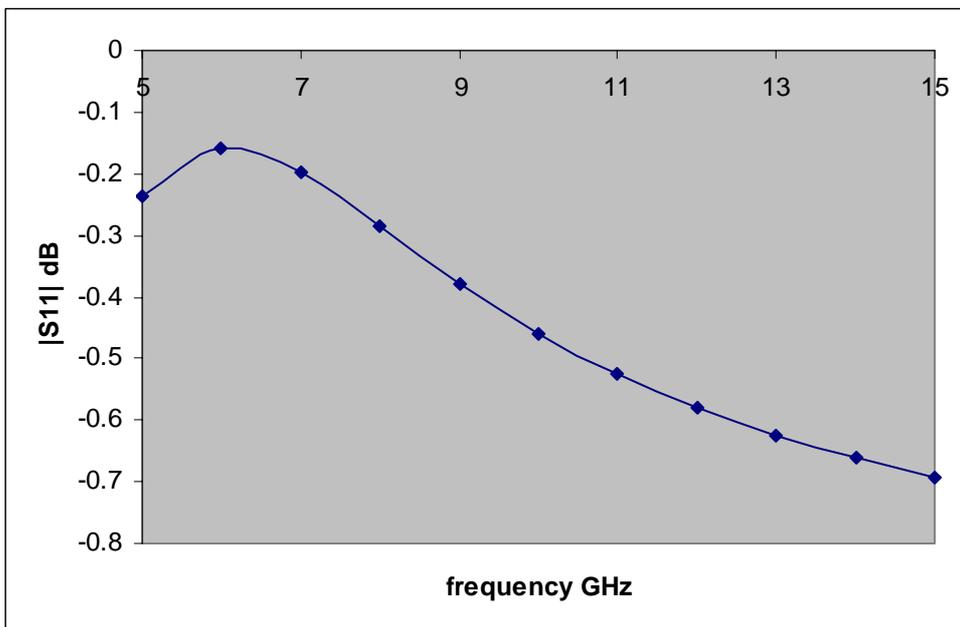
Fig. 4: Reflected signal from TIA input versus frequency.
