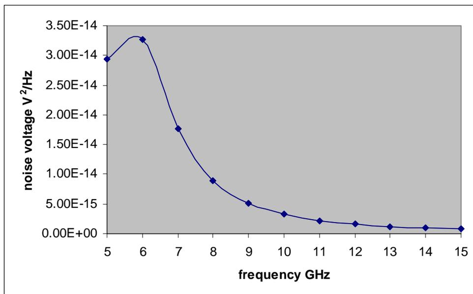
Fig. 10: Noise voltage after applying noise at TIA input.
