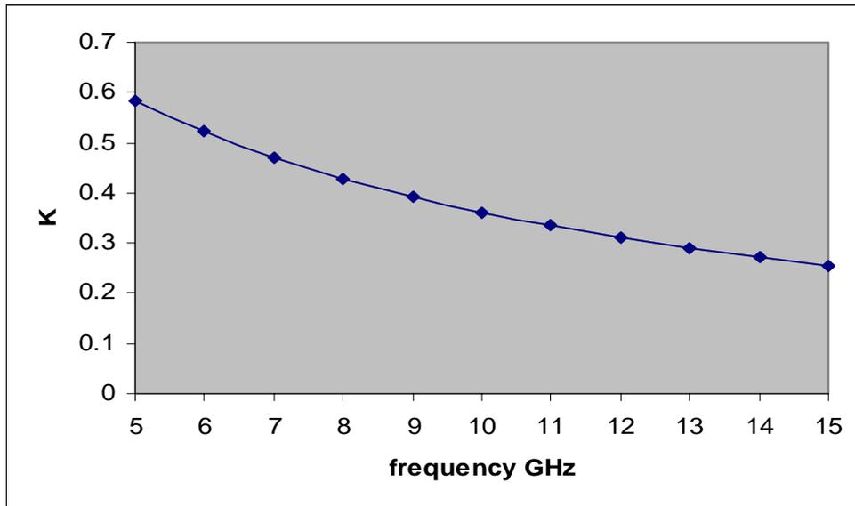
Fig. 5: TIA stability factor which indicated conditionally stable state at 10 GHz.
