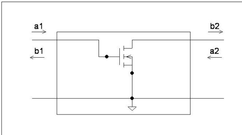
Fig.1: A transistor two port network.
