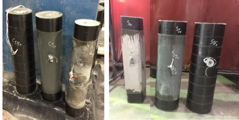
Fig. 4. Column specimens strengthened with RPC jacket and CFRP wraps (Hadi et al., 2018, a and Algburi et al. 2019, a)
