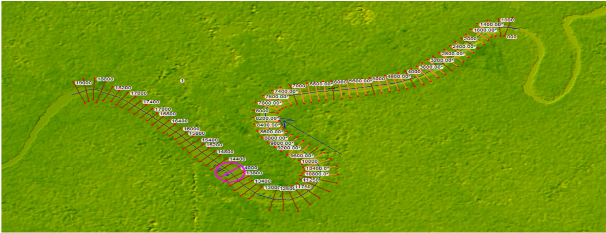
Figure 9. Editing Geometry in the HEC-RAS Models
