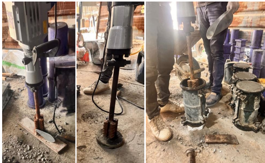
Fig. 5 hammer, rectangular head, and circular head are used for compacting RCC samples
