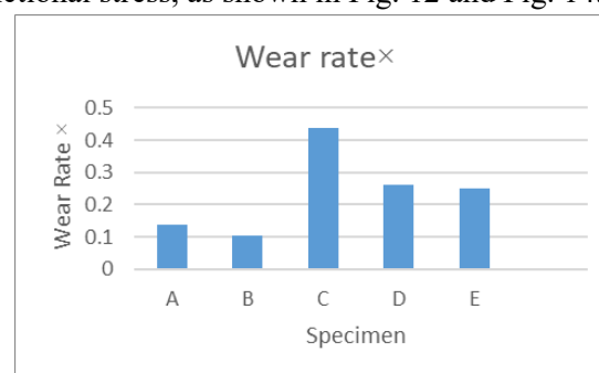
Fig. 12 The wear rate of the as-obtained specimens [higher power].
