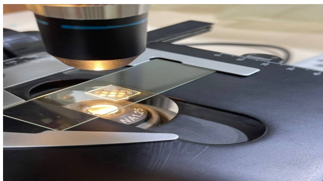
Figure 1. CR-39 detector with dimensions (1 \times 1) \text{ cm}^2 under optical microscope
