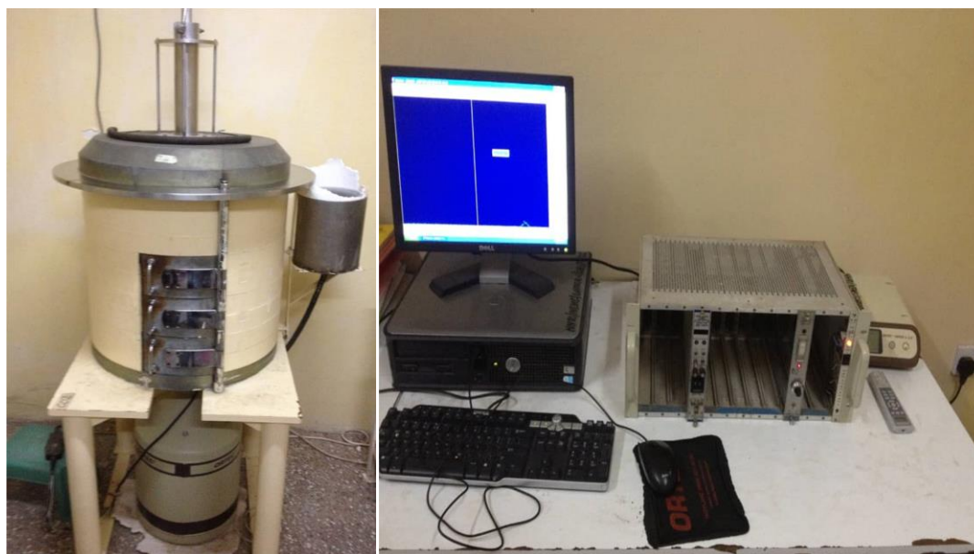
Figure. 1: The Radioactivity Measuring System
