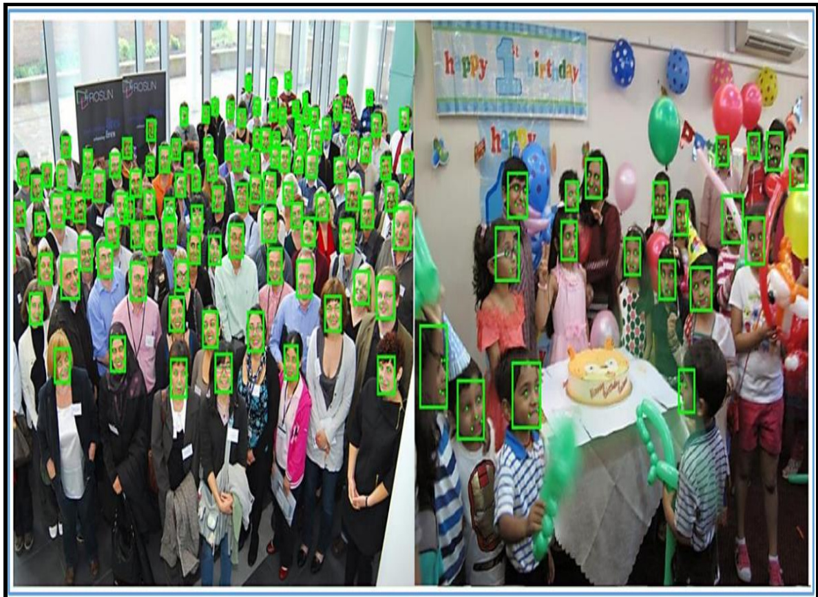
Figure 2: Face detection using the MTCNN face detector [15].
