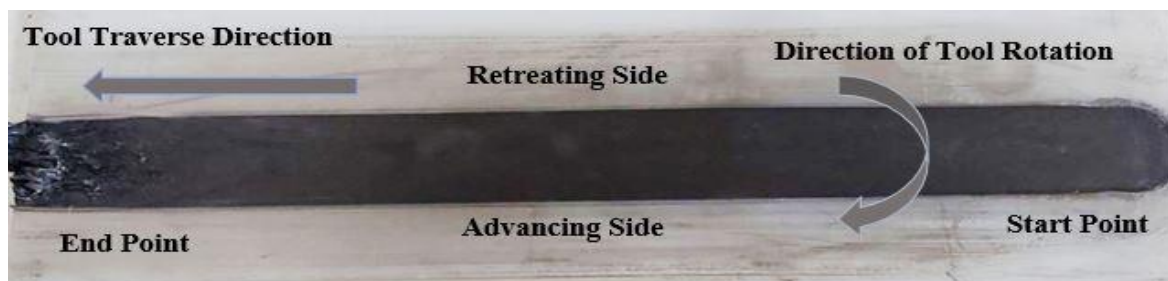
Figure 3. Prepared Sample by FSP
