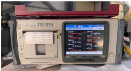
Fig. 5 Data logger used for control the loading and measuring the deflection in slab.
