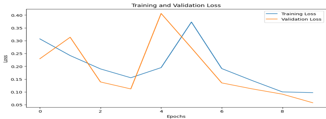
Fig. 4. Training and validation loss across 10 epochs, showing the model's steady improvement in minimizing error on both training and validation datasets. The training loss steadily decreases, while the validation loss shows initial fluctuations before stabilizing
