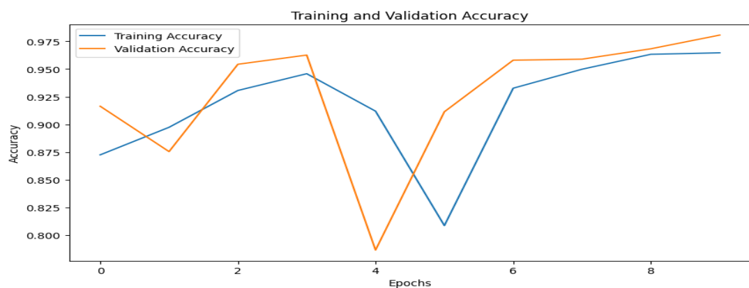
Fig. 5. Training and validation accuracy over 10 epochs, illustrating the model's increasing accuracy in both training and validation sets. Despite early fluctuations, the model achieves a high validation accuracy, stabilizing at around 97% by the final epoch.
