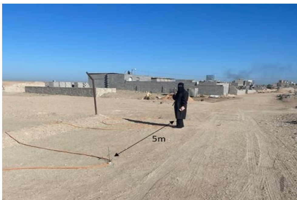
Figure 3: The spacing distance between electrodes is 5m.
