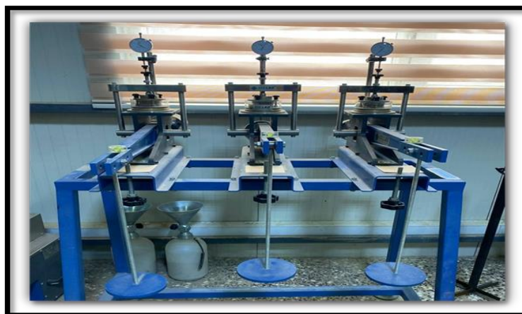
Fig. 2. Consolidation apparatus for collapsible test
