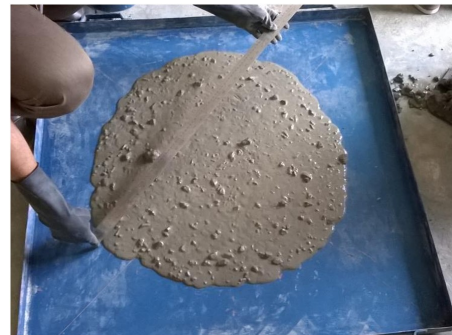
Figure 3. Slump Flow Test for SCC.
