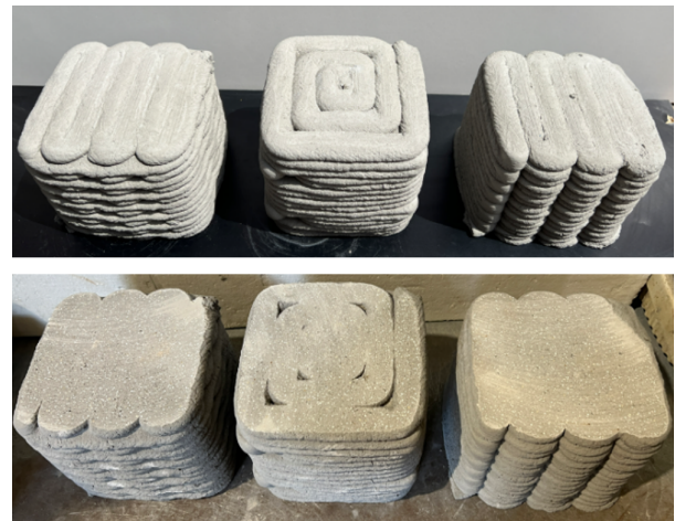
Figure 11. 3DPC cubes before and after surface smoothing.
