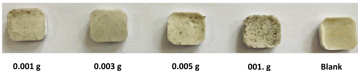
Fig. 8. Photograph of blank melamine formaldehyde tablets loaded by (0.001, 0.003, 0.005, and 0.01 g) of wp-GO powder.
